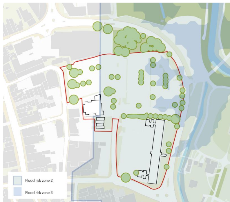
Figure 6: Flooding constraints at Old River Lane
