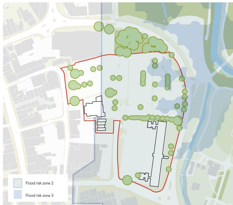
Figure 5: Flooding constraints at Old River Lane
